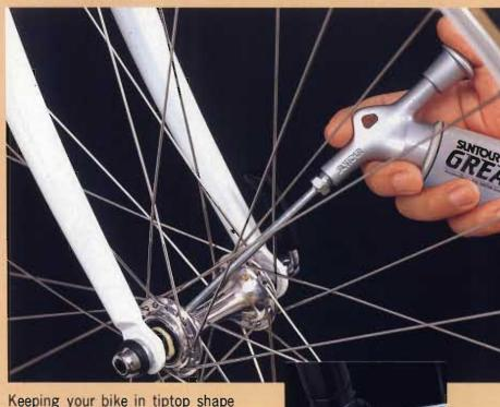
Keeping your bike in tiptop shape has never been easier. The new WTB/SUNTOUR Grease Guard System lets you clean and lube your hub, bottom bracket, headset and pedals in just a matter of seconds. It's simple. As you inject new WTB/SUNTOUR grease into the convenient injection ports, you purge out the used and contaminated grease. In just seconds you've overhauled your bike's most critical parts: the hub, bottom bracket, headset and pedal bearings. There' s no better way to keep your bike
