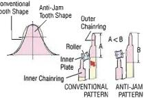
Specially shaped teeth, combined with a specially profiled side pattern on the chainrings, help the chain shift down without hanging up and jamming. Mounted to the outer chainring is an anti-jam pin, which keeps the chain from getting jammed between the crank arm and the chainring.
